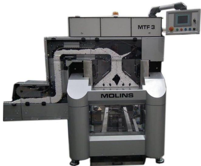
The MTF 3 is a new Molins Mass Flow Tray Filling Machine. Designed to address all the needs of the cigarette and filter making industry, using reliable proven features of the very successful MTF2. The MTF 3 is PLC controlled with all motor speeds and tray adjustments made on a touch screen.
