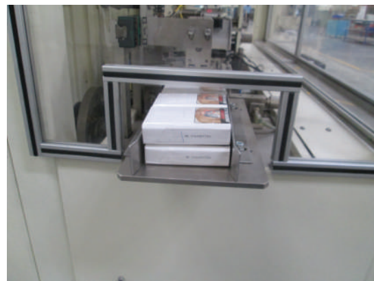
Packet collator at exit to deliver 2 high stack
